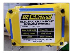
Tape up the three (3) sides of the cover of the OZ Electric Chain Hoist as shown.
