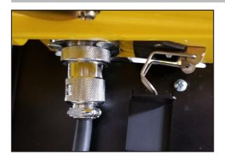
Insert and tighten the control plug to the connector on body as shown.
