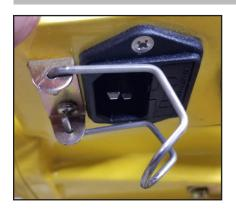
On the existing power cable connector on the body of OZ Electric Chain Hoist, flip retaining latch as shown.
