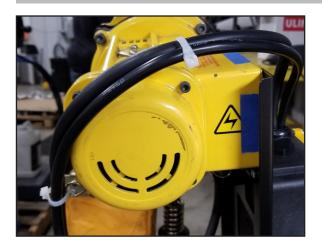
It is advised to tie-up the wiring with zip ties as shown to reduce the possibility of damage.
