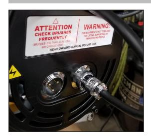
Insert and tighten the 5-pin male connector of the receiver cord into the 5-pin female connector on hoist body. It is advised to tie-up the wiring with zip ties to reduce the possibility of damage.
