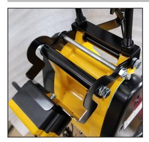
Remove the cotter pin and nut from the mounting bolt. Ensure that the bracket arms of the receiver are on the outside of the bracket on the hoist itself. Insert the mounting bolt, reinstall the nut and cotter pin as shown below.
