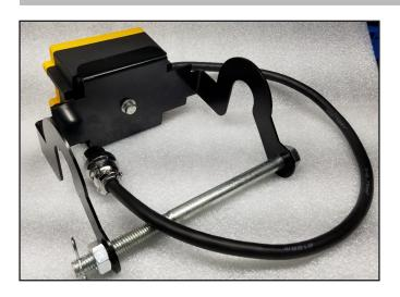
Mount the bracket to the receiver as shown. Do not over-tighten the 10mm hex head bolt as it may damage the housing.
