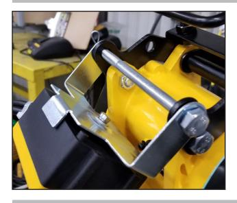
Remove the cotter pin and nut from the mounting bolt. Ensure that the bracket arms of the receiver are on the outside of the bracket on the hoist itself. Insert the mounting bolt, reinstall the nut and cotter pin as shown below.
